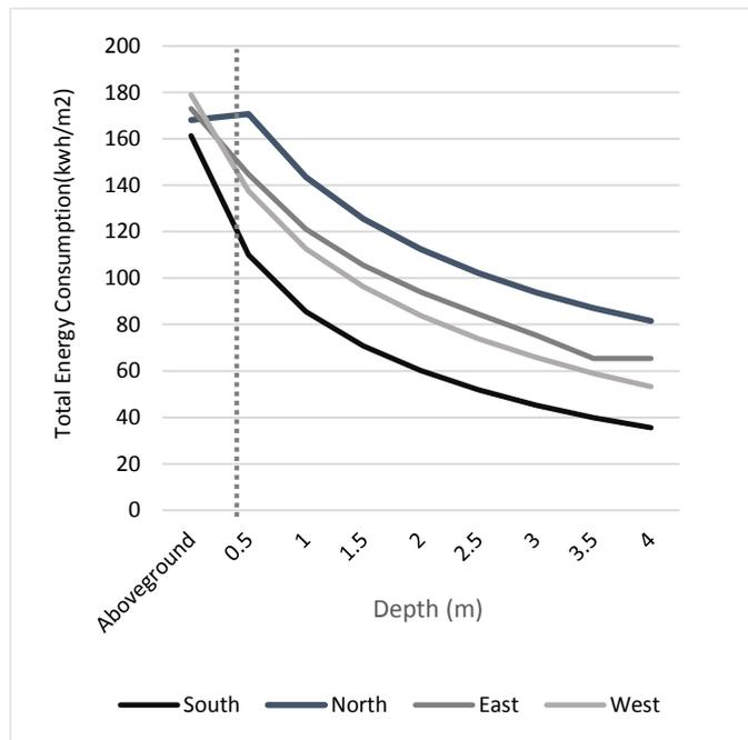
Fig. 3. Total Energy Consumption in different orientation
