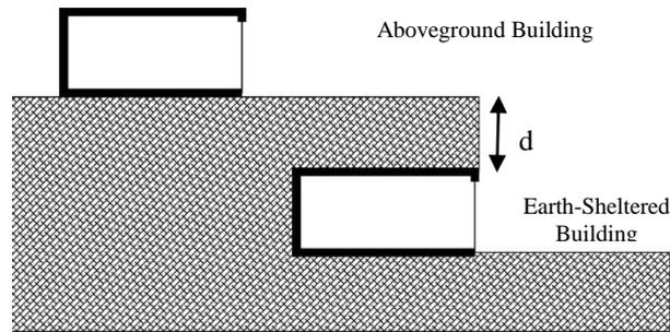
Fig. 2. Situations of models in Different Depth during Simulation Procedure
